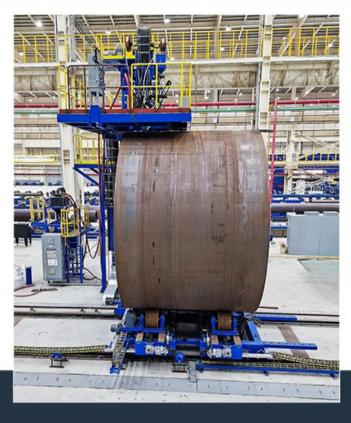
OSL's OSTrack-NG system was designed for narrow gap and semi narrow gap welding applications.
