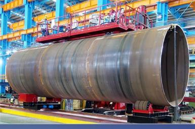
OSL staff worked on the world's first monopile production line over twenty years ago, where the scanning spot sensor technology and multipass software with memorization and replay were first applied together for semi narrow gap welding.
